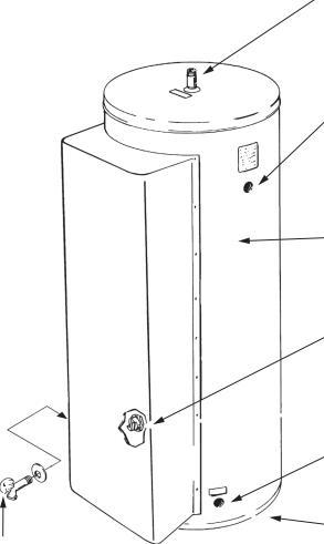
Drain valve leakage could be from the valve itself. Either correct the problem or replace the valve\*. To check for leakage where threaded portion enters tank, insert Q-tip or similar absorbent material between jacket opening and valve to swab spud area. Remove valve\* if leak is indicated and repair with pipe joint compound.
