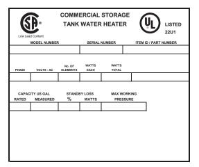
Figure 2. Example Rating Plate
