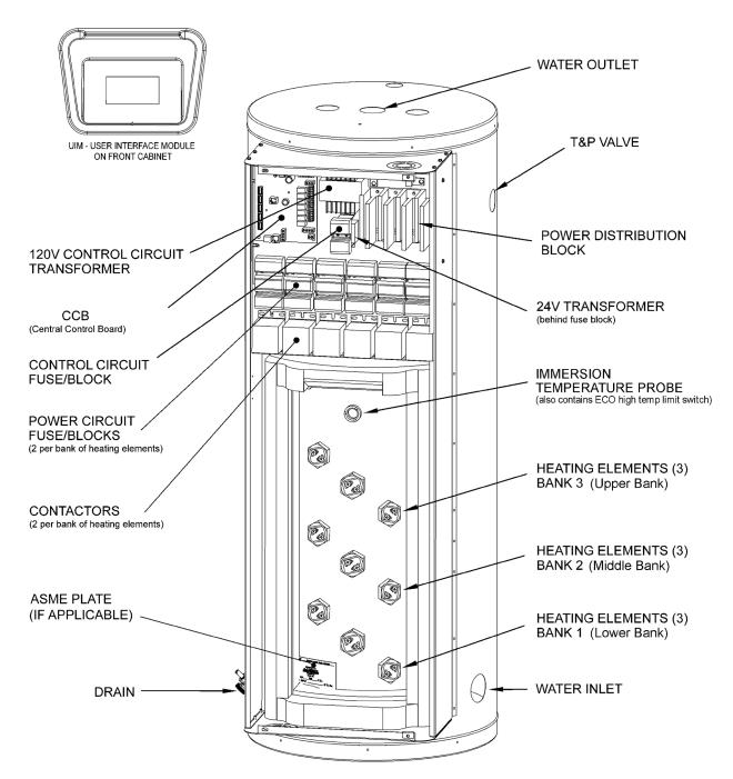
**Figure 3. Electronic Control Models**
