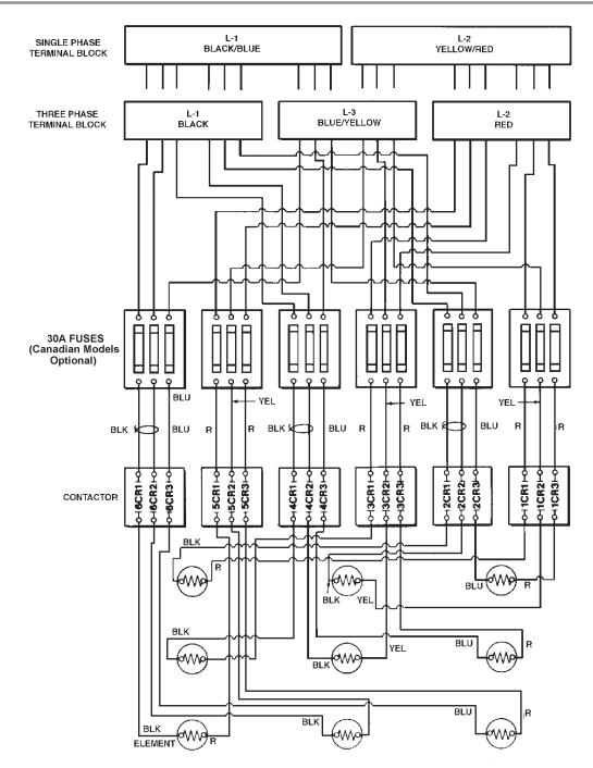
Figure 10. Nine-Element Single- and Three-Phase Power Circuits
