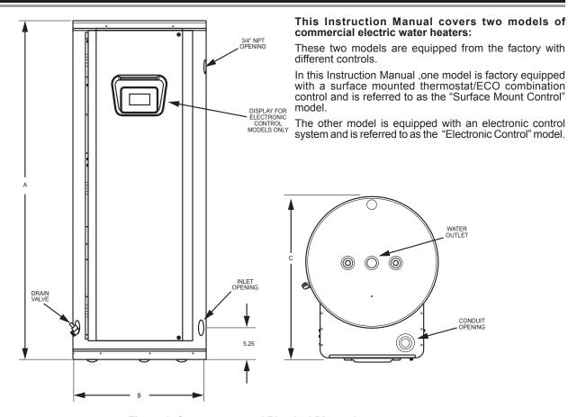
Figure 1. Components and Physical Dimensions
