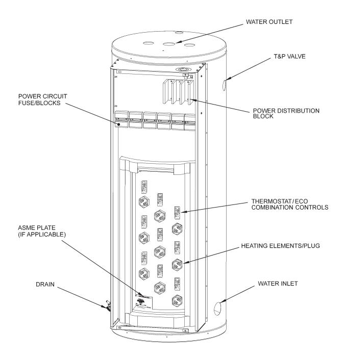
**Figure 4. Surface Mount Control Models**
