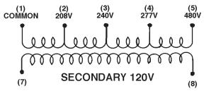
Figure 6. Transformer Secondary Loop
