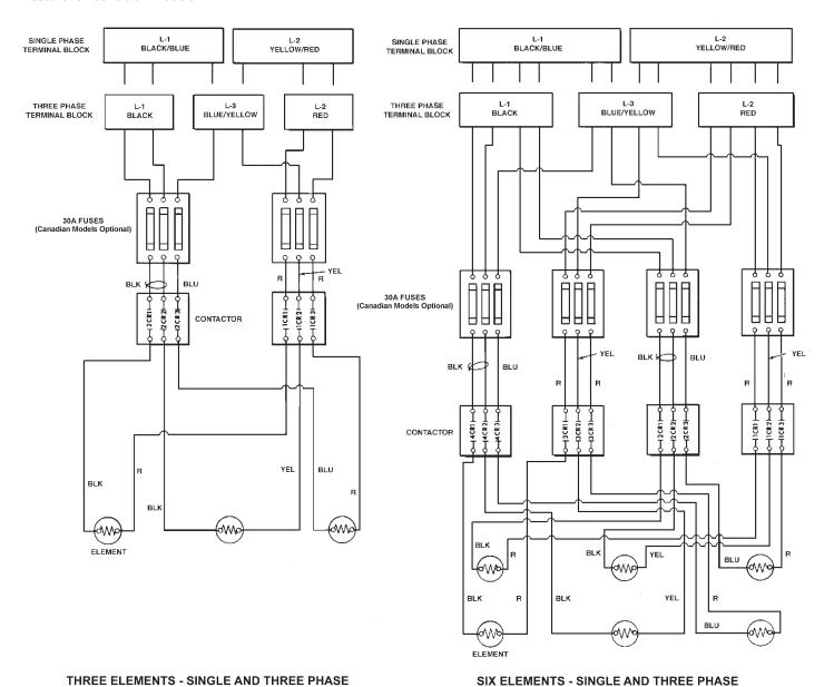
Figure 9. Three- and Six-Element Single- and Three-Phase Power Circuits
