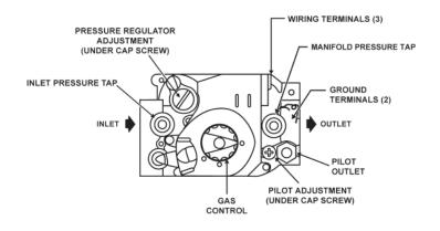
FIGURE 23. ADJUSTING PILOT FLAME
