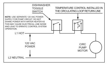
FIGURE 6. CIRCULATING PUMP WIRING DIAGRAMS FLOW SWITCH (NOT SUPPLIED)
