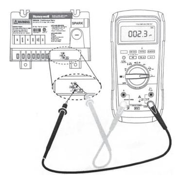
FIGURE 19. MEASURING PILOT FLAME CURRENT WITH MICRO-AMMETER.
