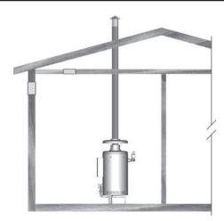
FIGURE 10. OUTDOOR AIR THROUGH ONE OPENING
