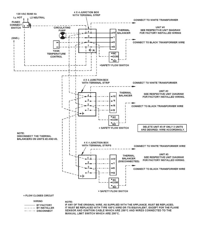
FIGURE 28. CER - TEMP 80 - 2 OR 3 UNIT INSTALLATION CONNECTION DIAGRAM - FOR HOT WATER SUPPLY APPLICATION
