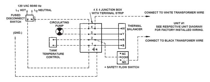
FIGURE 26. CER - TEMP 80 - 1 UNIT INSTALLATION - FOR HOT WATER SUPPLY APPLICATION
