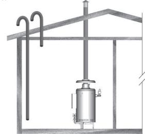
FIGURE 12. OUTDOOR AIR THROUGH TWO VERTICAL DUCTS
