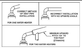
FIGURE 14. VENT PIPE INSTALLATION
