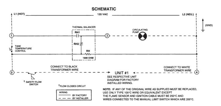
FIGURE 27. SCHEMATIC: CER - TEMP 80 - 1 UNIT INSTALLATION - FOR HOT WATER SUPPLY APPLICATION
