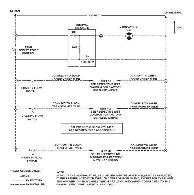
FIGURE 29. CER - TEMP 80 - 2 OR 3 UNIT INSTALLATION SCHEMATIC DIAGRAM - FOR HOT WATER SUPPLY APPLICATION
