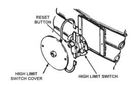
FIGURE 5. MANUAL RESET HIGH LIMIT SWITCH
