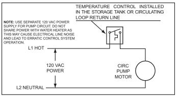
CIRCULATING PUMP WIRING DIAGRAM DISHWASHER LOOP WITH TOGGLE SWITCH
