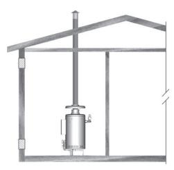
FIGURE 9. OUTDOOR AIR THROUGH TWO OPENINGS
