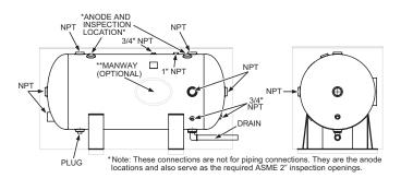
FIGURE 4. HORIZONTAL TANK.
