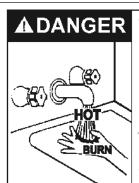
Water temperature over 125°F (52°C) can cause severe burns resulting in severe injury or death.
