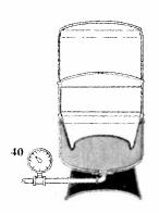
2. As water enters the tank, the air above the diaphragm is compressed and its volume is reduced by the volume of water that enters.
