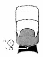
4. The pressure in the air chamber forces water into the system when a demand occurs without causing the pump to operate immediately. Pressure in the chamber finally drops to the pump cut-in pressure, the pump switch activates the pump and repeats the filling cycle.
